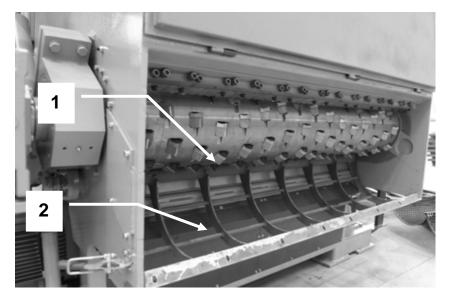
The rotor is accessible after opening the machine door and removing the screen.
